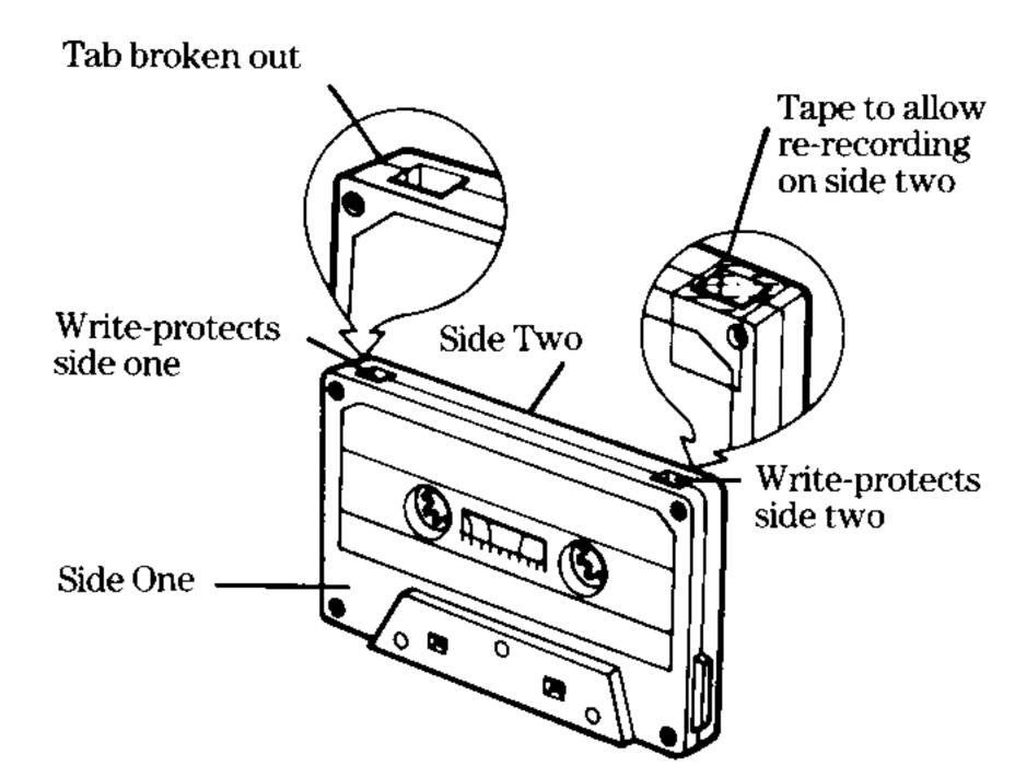
**Note:** If you need to record on a tape that has a tab missing, place a piece of cellophane tape over the tab opening before you record a file.
